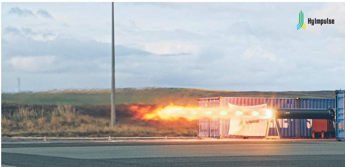
Figure 3 Firing of the SR75 motor during a qualification test at the HyImpulse test facility on the Shetland Islands
